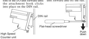
Be sure that the top and bottom faces of the unit are facing the correct direction and the unit is installed in a vertical position. Incorrect installation may cause overheating.
